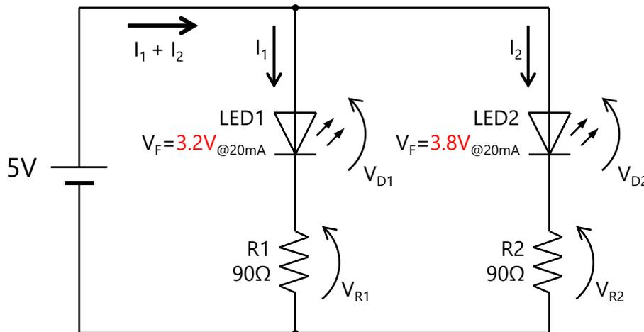
Figure 1. Circuit Diagram
