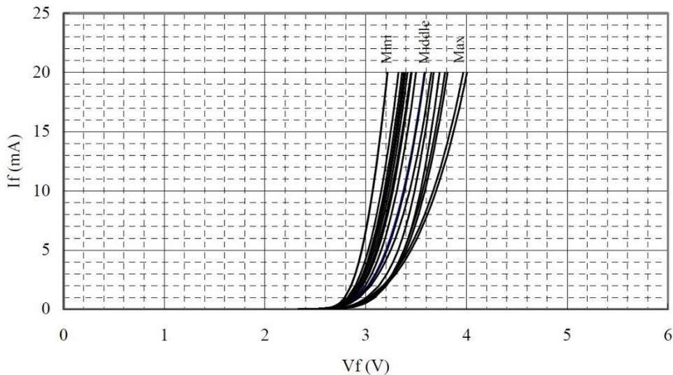
Figure 2. Forward Voltage - Forward Current
